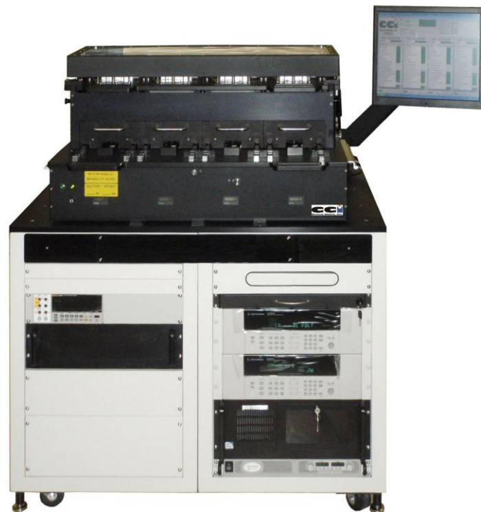
Test stand and fixtures to test four parts at a time
