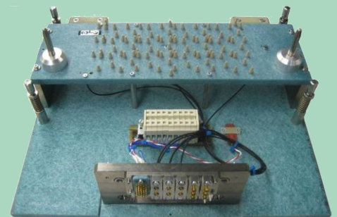
Top fixture manufactured using high temperature materials
