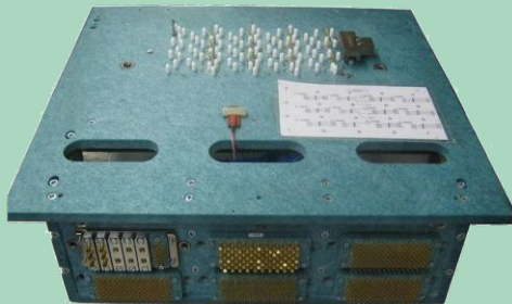
Bottom fixture manufactured using high temperature materials
