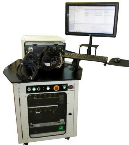
Example cabled ITA fixture
