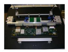
Pneumatic Side access unit with mechanical hold down unit to hold customer product to specific level Allowing for precise engagement of connectors.
