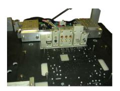
Side access Unit close up of mating contacts that are inserted into connectors for functional through connector testing of product.
