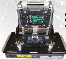
Functional fixture where the unit under test is plugged into an interposer board mounted on probe plate.
