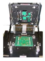
Interposer board shown mounted on top of probe plate in bottom of fixture. Interposer board has clearance holes drilled through it for the probe field.
